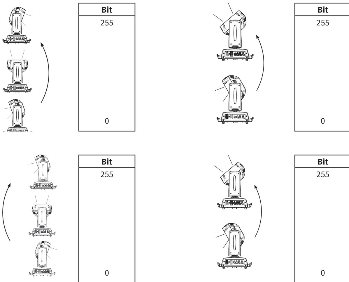
Operation with option InvertPan, GOn (Tilt conventionally represented at 35 bit and option Invert Tilt, GOff)
